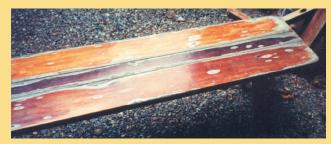
System Three Clear Coat<sup>™</sup> resin is an excellent barrier to both liquid and vapor moisture. It is easy to apply with a brush or a roller and contains no hazardous solvents. It will cure to a tough, clear, high-gloss film which will waterproof the wood. But the epoxy film, because it is clear, does not protect the wood from sunlight. In addition, exposure to the sun will dull, darken, and eventually degrade an epoxy coating. To avoid ultraviolet light
